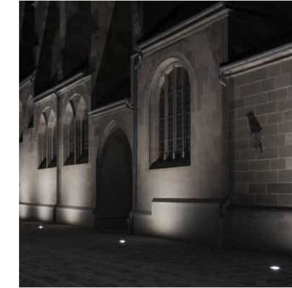
Recessed Uplights in Floor Highlight Structure & Provide indirect light
